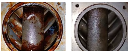
Oil-injected screw compressor: Before and after treatment with SludgeGuard
