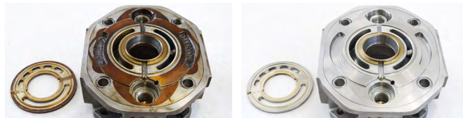
Hydraulic system components: Before and after treatment with SludgeGuard
